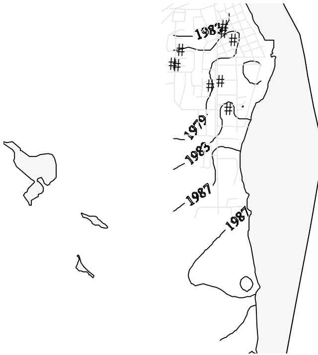
Figure 13: Locations where total coliform bacteria were detected in samples from domestic wells at Site 3. Contours show year in which the domestic wells were drilled.
